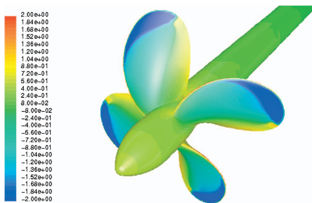
Fig. 11 (Color) Pressure coefficient contours on backside at J=0.2 and \sigma=2.0
